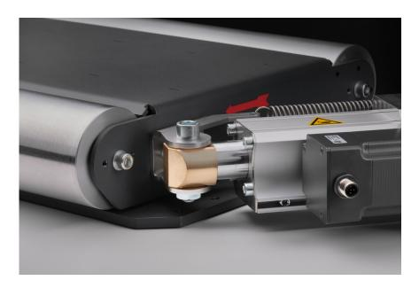
BST solutions enable battery manufacturers to meet the highest quality requirements in an economical way. With its newly developed, high-performance drive with repeat accuracies of 10 m, the ultra-precise web guiding system, FRAMEGuide Pro, ensures high-precision guiding results in every application.
