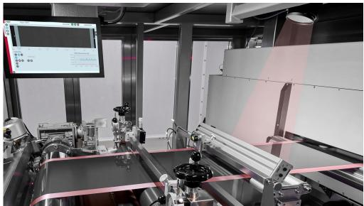
In battery production, the smallest irregularities lead to rejects. This is where BST COATINGControl delivers the decisive competitive advantage by increasing plant efficiency: The system uses high-precision measurement and control technology to ensure perfect coating geometry on the front and back.
