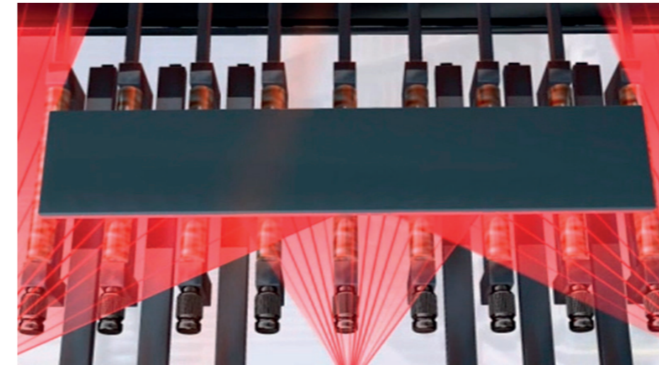
Functional principle of the slab position measurement on the roller table
